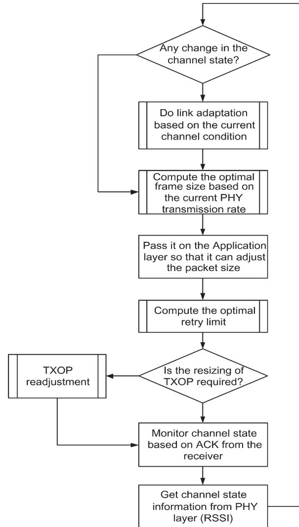
Fig. 10. Cross-layer algorithm that is performed at the MAC layer.
