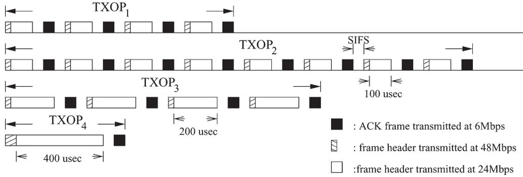
Fig. 4. Example 1—Selection of TXOP limits. Given that SIFS = 16  $\mu$ s, frame header size = 34 B, and ACK frame size = 14 B in the IEEE802.11a standard, we have TXOP<sub>1</sub> = 619.6  $\mu$ s, TXOP<sub>2</sub> = 1255.2  $\mu$ s, TXOP<sub>3</sub> = 1019.6  $\mu$ s, and TXOP<sub>4</sub> = 512.5  $\mu$ s.<sup>1</sup>
