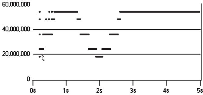
Fig. 11. Link adaptation algorithm for IEEE 802.11a.
