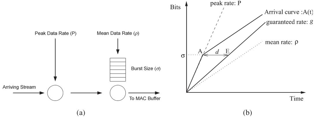
Fig. 2. Token bucket policer and the arrival curves. (a) Token bucket representation of admission control. (b) Arrival curve and calculation of guaranteed rate.
