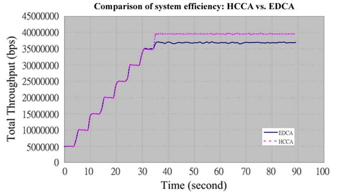
Fig. 6. Comparison of system efficiency, in terms of the total throughput, between the HCCA and the EDCA.<sup>3</sup>
